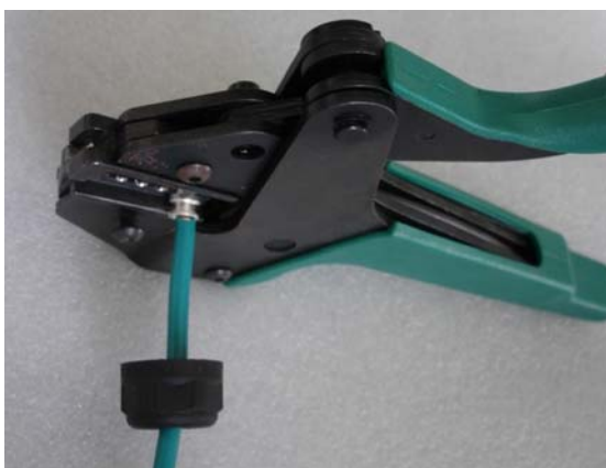
Figure 3-8 connect step No.3
