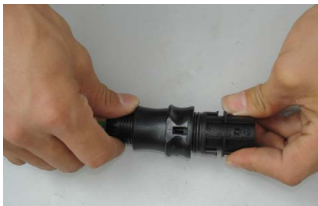
Figure 3-14 put the coat to the terminal Where, put the connector to the GCI-5K.
