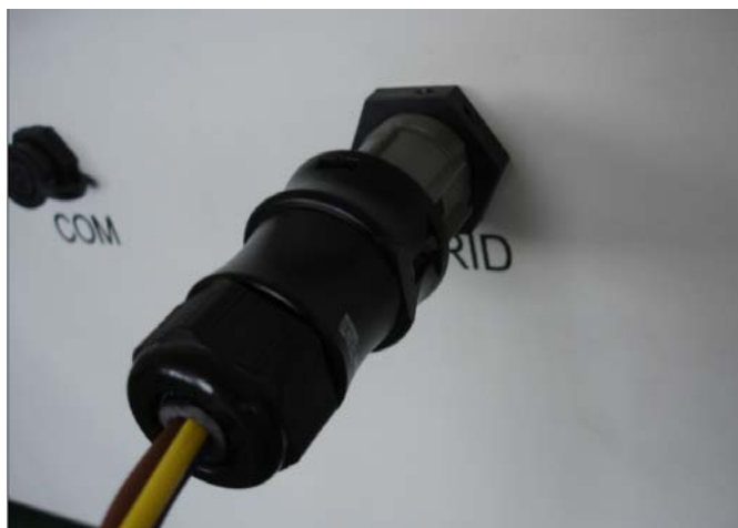
Figure 3-15 connect the terminal to GCI-5K
